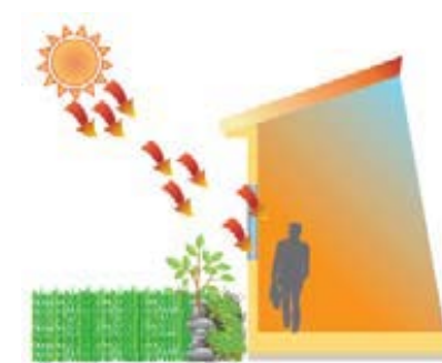
In cooler climates, a high SHGCw (as illustrated) is beneficial for north facing windows during winter, however shading will be required in summer to prevent unwanted solar heat gain. In hot climates, a low SHGCw is always ideal.
