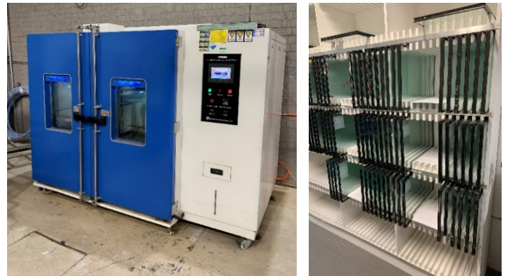
Figure 1: Long term accelerated weathering testing chamber and facilities
