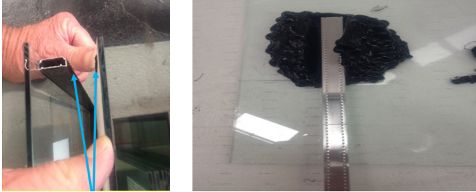
Figure 2: Testing of sealant adhesion
