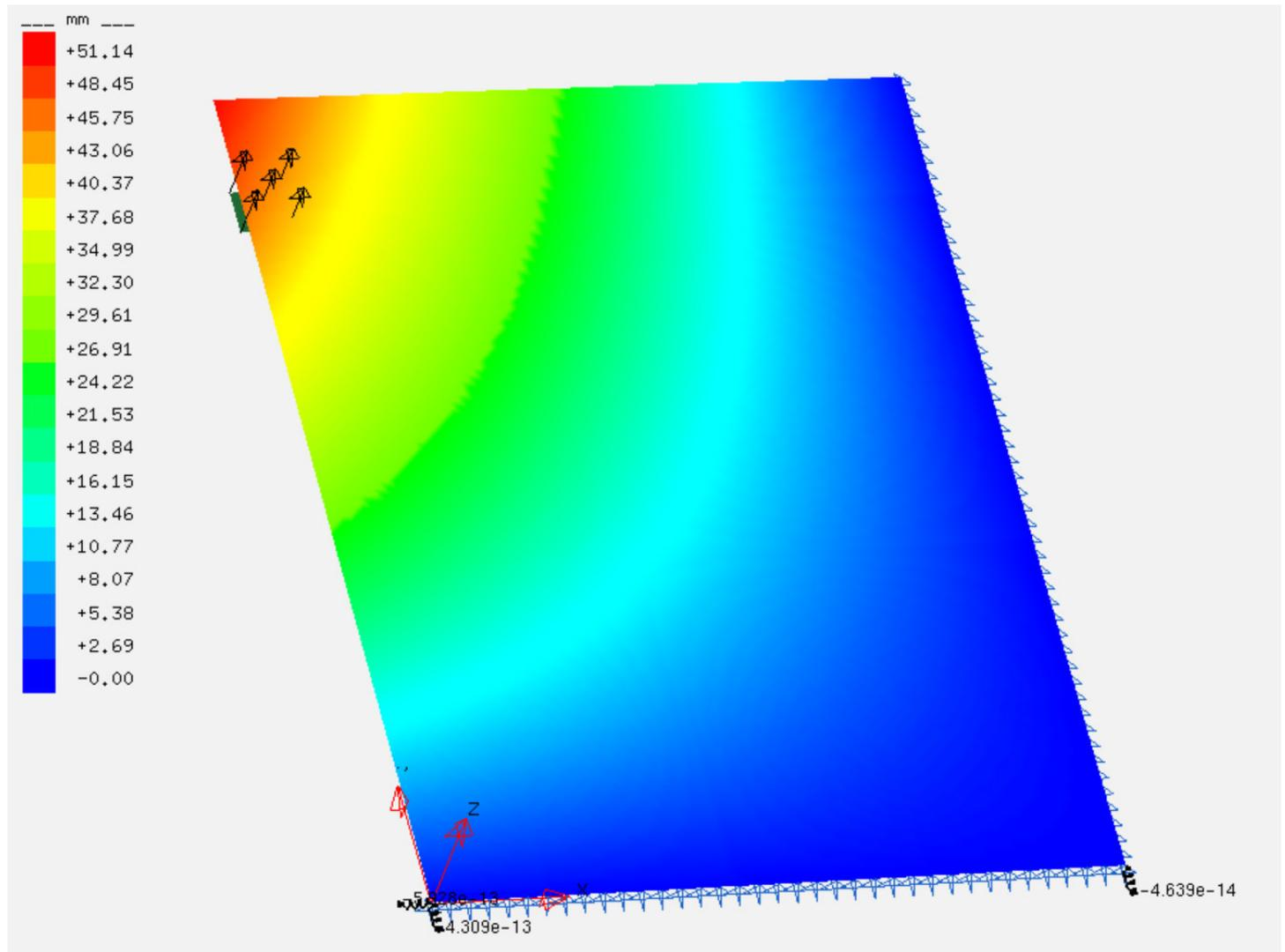
**Figure A** 10 mm thick panel showing about 50 mm deflection
