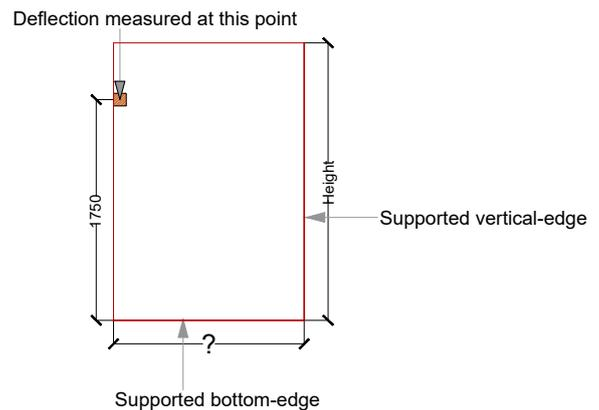
**Figure 1** Load location for shower panel supported on two adjacent edges.
